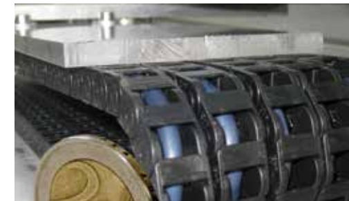
Control cable CF98.05.04 tested in e-chain®. More than 138 million strokes with a bending factor of 3.2 x d
