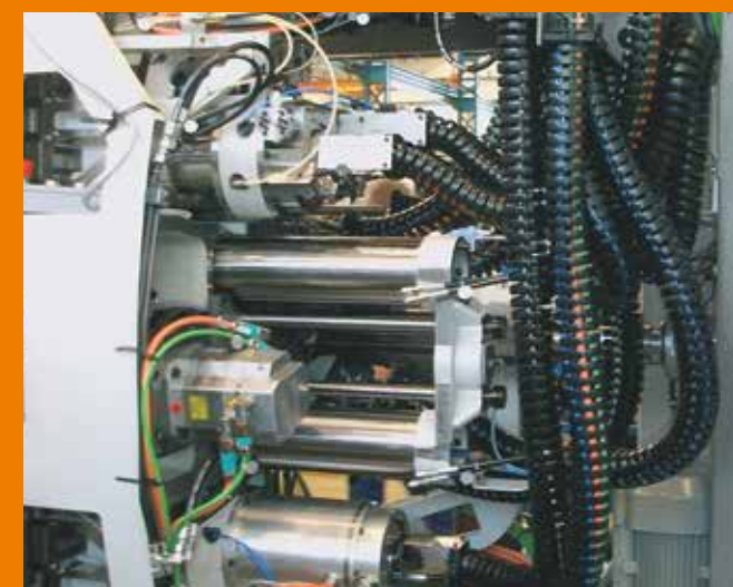
triflex® TRL - lightweight, for quick cable removal
