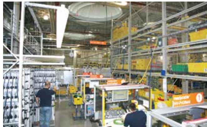
Computer-based high-voltage testing and inspection of all assembled cables
