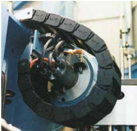
Rotary motion with a standard igus® e-chain®
