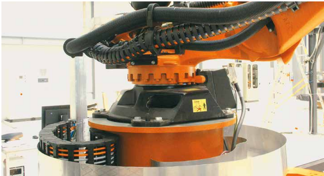
System E2 medium with 360° RBR rotary motion on a robot
