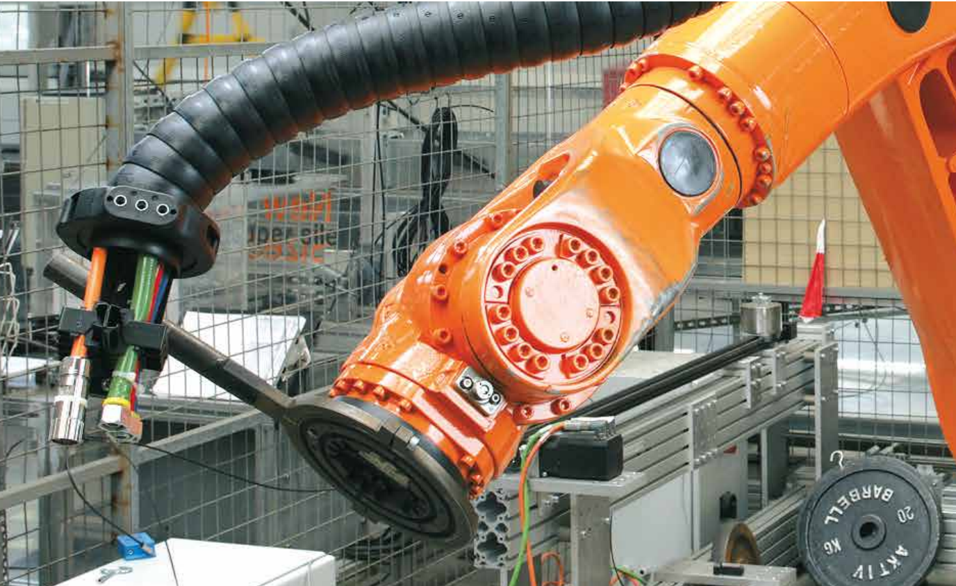
Individual strain relief for every cable allows security and easy replacement
