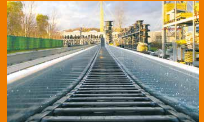
Long travel test field - 125 m travel length, speed 300 m/min
