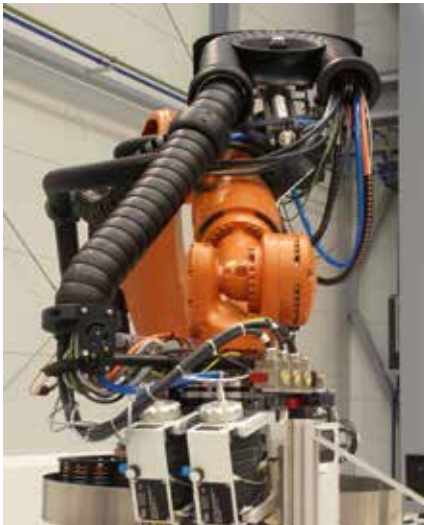
igus® chainflex® cables in application of a multi-dimensional moving e-chain® trifix R for 6-axis robots.
