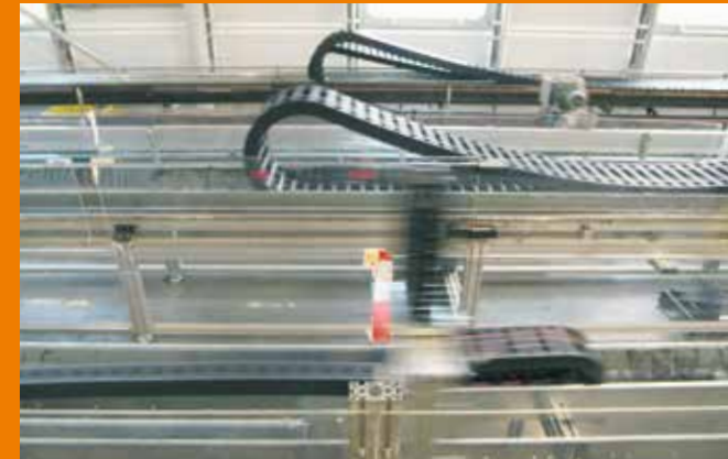
Speed up to 10 m/s and acceleration up to 200 m/s 2 are tested by igus ®
